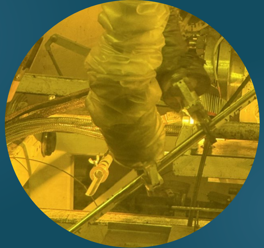
Handling and packaging in hot cell
