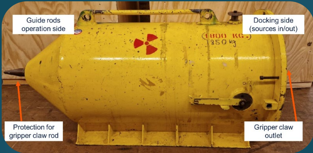
Co-60 source transportation flask (1850 kg)
