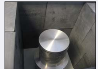
Pic. 3: 3" NaI detector used for fresh samples
