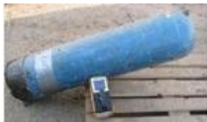
Water filter 0.3 microSv/h, 2.2-3 Bq/g Ra-226 Total weight: 30 kg, NORM 28 kg
