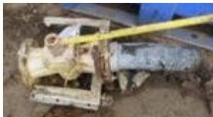
Very thin scale in an industrial equipment detail 1 microSv/h, 1000-1500 Bq/g Ra-226 Total weight: 5 kg, scale 20 g
