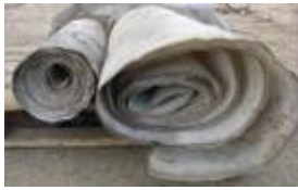
Filter cloth 14 microSv/h, 130-180 Bq/g Ra-226 Total weight: 20 kg/piece
