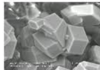
Morphology of the AlN powders with perfect crystallinity
