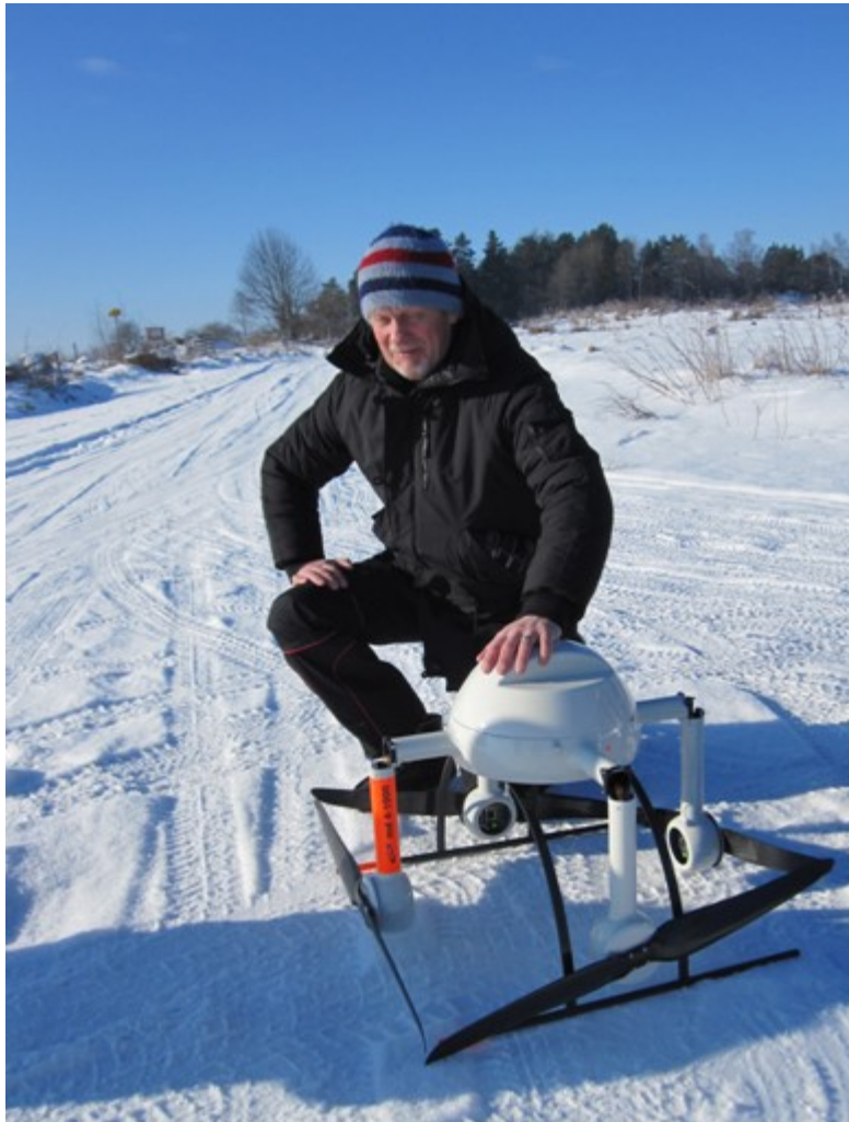
Figure 2 Third author by the microdrone illustrates the size. The microdrone's rotor arms are folded for transportation. Photo by first author.
