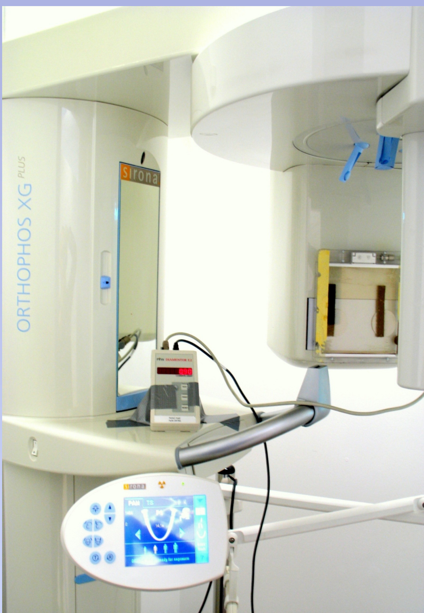
Picture 1 A translucent transmission ionization chamber is connected to a DAP meter (Diamentor E2, PTW-Freiburg, Germany)
