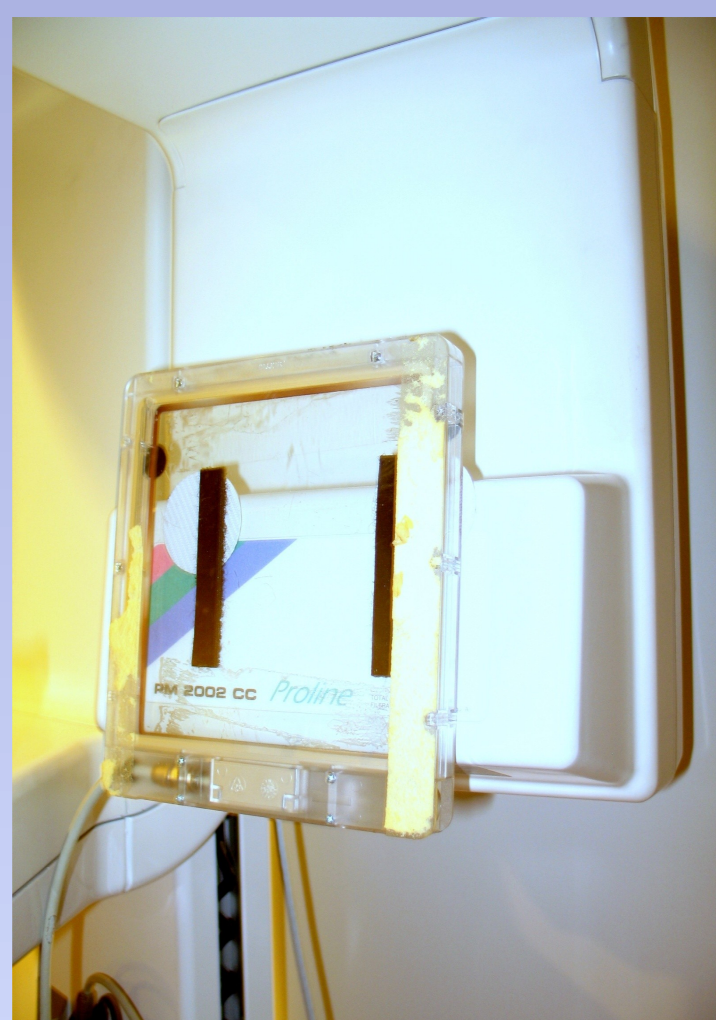
Picture 2 The ionization chamber was attached directly in front of the exit slit of the x-ray tube
