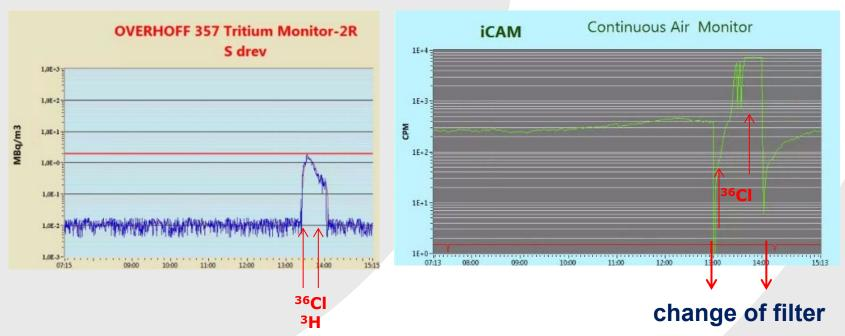
Filter from air-monitor dissolved and <sup>36</sup>Cl identified.
